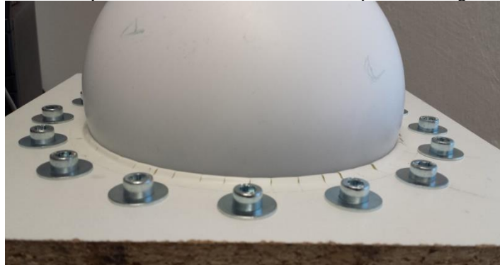
Figure 11: Sample of Wacker R360 inflated to an apex stretching of 135%
