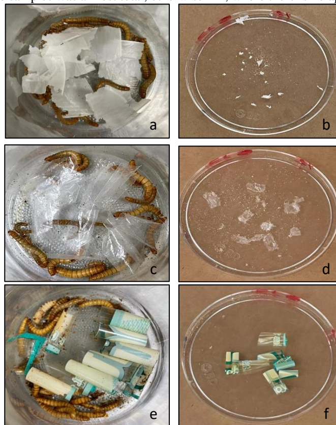
Figure 2. Degradation of CPE, LDPE, d2wPE with UV pretreatment after 7 days of experimentation (a, c and e). In a and c, the bites of the larvae began to be visible. In case e, only the effects of change of shape and color in the sample are appreciated. Degradation of CPE, LDPE, d2wPE with UV pretreatment at 56 days of experimentation (b, d and f). In b and d, the mass loss of the samples was almost total, otherwise in f, where there is no apparent degradation.
